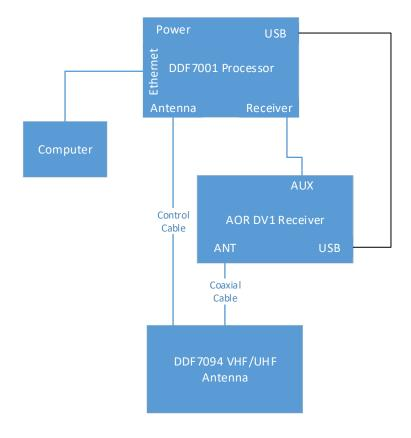
Figure 1: Wiring Diagram for Doppler Direction Finder with AOR DV1 Receiver
