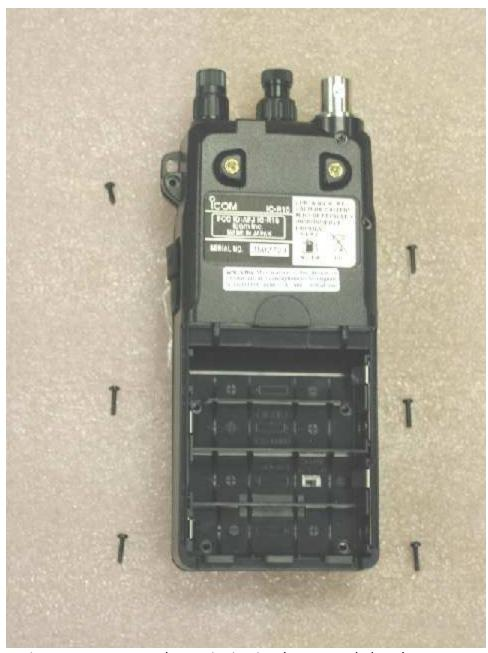
3. Carefully open the receiver case to expose electronic circuitry (see second photo).
