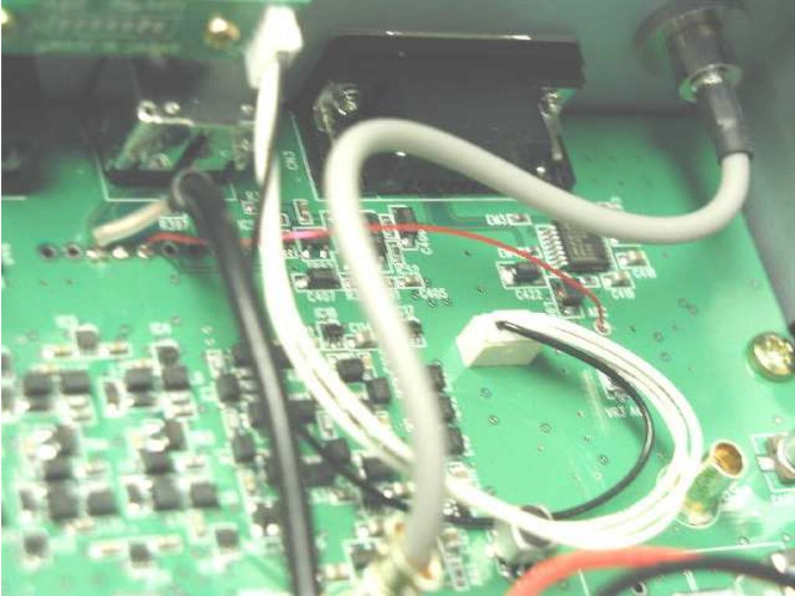
Reattach the loudspeaker and reassemble the shield plate and top cover.
