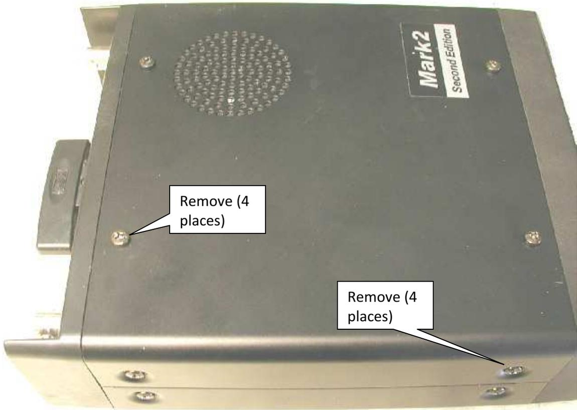
Now remove the 6 screws that retain the shield plate as shown. After lifting out the shield plate, unplug the loudspeaker connector.
