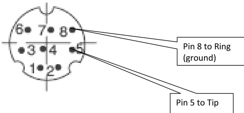
After reassembling the Mini-DIN connector, you may find that because of the thickness of the rear cover on the AR8600, the mating plug will not mate with the recessed connector pins sufficiently to make a reliable connection. This can be easily corrected by using a single edged razor blade to trim the soft outer protective cover on the plug about 1/8 inch back from the hard plastic insulator as shown below.
